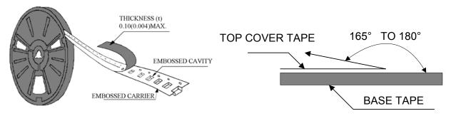
The force for peeling off cover tape is 10 grams in the arrow direction.
