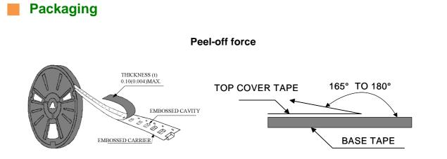
The peel off force of cover tape is 10 to 70 grams in the arrow direction.
