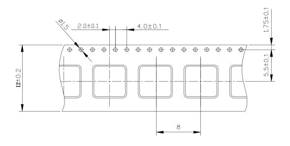
(6)-2 TAPING DIMENSIONS (mm)
