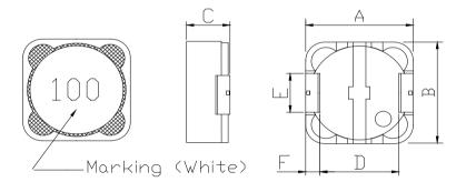
A: 10.3 Max. mm B: 10.3 Max. mm C: 4.00 Max. mm D: 6.4±0.3 mm E: 4.6±0.2 mm F: 1.7±0.2 mm
