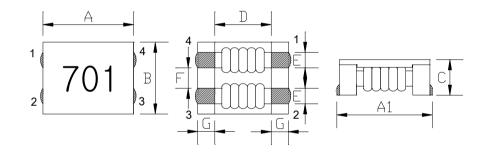
A: 7.0±0.5 mm A1: 7.5±0.5 mm B: 6.0±0.5 mm C: 3.8Max. mm D: 3.5Typ. mm E: 1.5±0.3 mm F: 1.5±0.3 mm G: 1.75±0.2 mm
