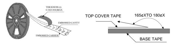
The peel off force of cover tape is 10 to 70 grams in the arrow direction.
