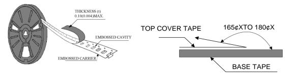
The peel off force of cover tape is 10 to 70 grams in the arrow direction.
