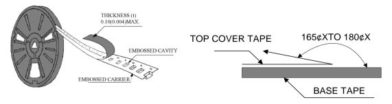
The peel off force of cover tape is 10 to 70 grams in the arrow direction.
